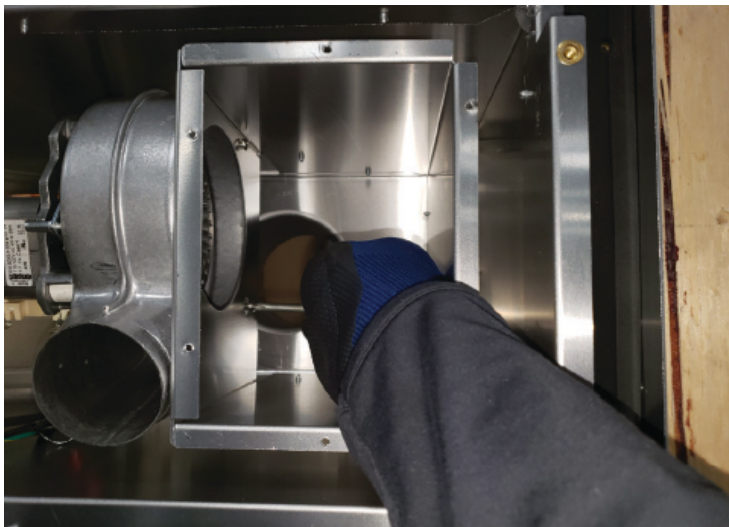
Figure 8.6 - Remove (3) Screws Securing Fan Assembly
