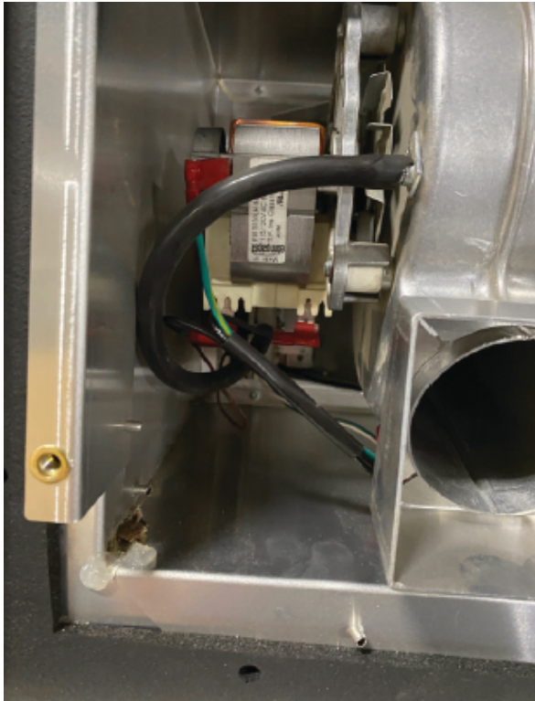
Figure 8.8 - Screws Securing Vacuum Switch Bracket
