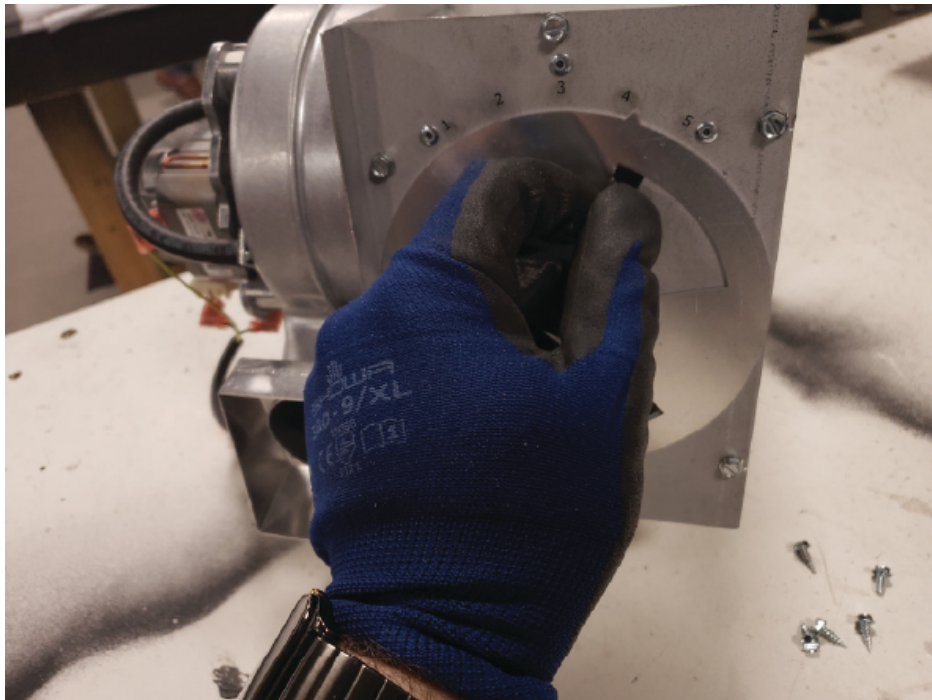
Figure 2.5 - Adjust the Draft Bypass
