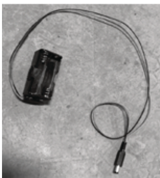
Figure 9.1 - Battery Back-up and Barrel Jack
