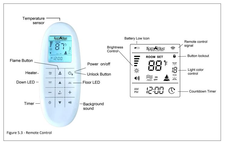
Note: The remote will go into safe mode after 60 seconds of not being used. Press the "unlock" button on the remote to unlock the remote before use. When you press the "unlock" button the remote screen backlight will turn on.
