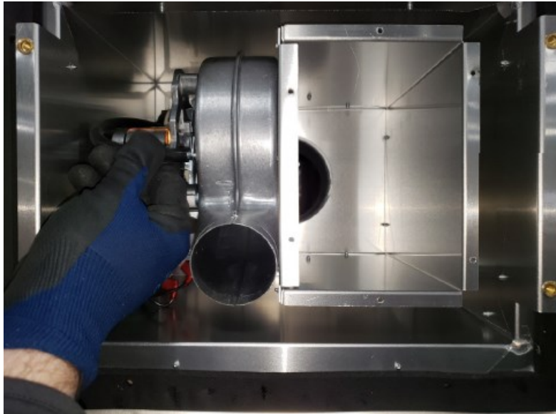
Figure 8.5 - Remove Vacuum Tube
