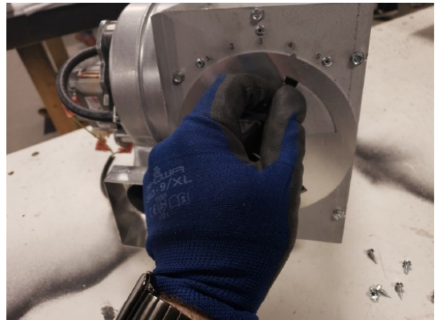
Figure 2.5 - Adjust the Draft Bypass
