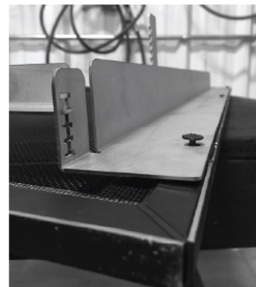
Figure 5.9 - Screen Barrier Louver Adjustment
