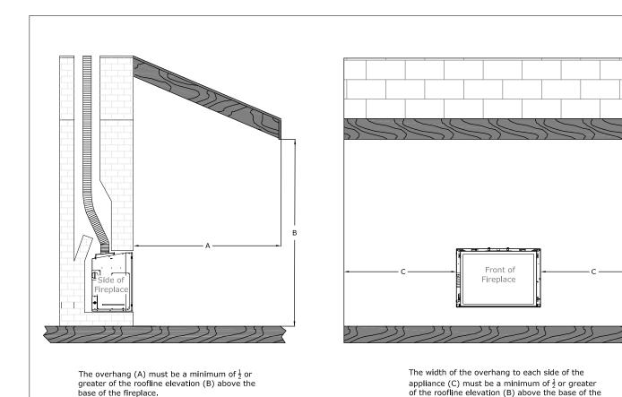
base of the fireplace, the overhang (A) must be 5' or greater and the width of the overhang to each side of the fireplace (C) must be 5' or greater.
