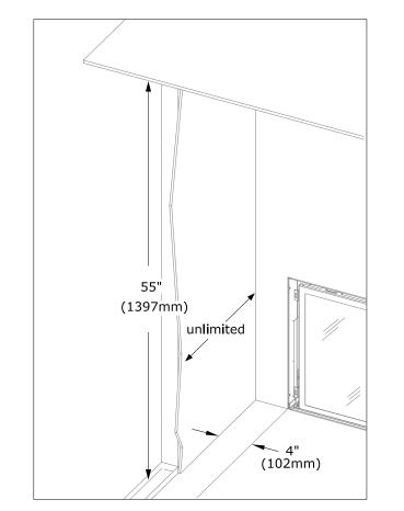
Figure 8.1, Clearance to sidewall
