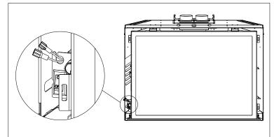
Figure 11.1 Back-up Battery Connection
