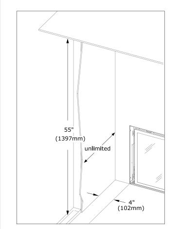
Figure 8.1, Clearance to sidewall
