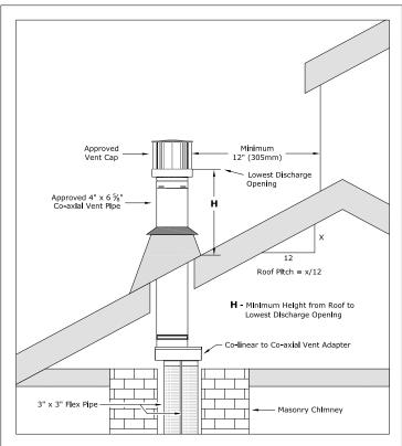
Figure 4.3, Co-linear to Co-axial Vertical Termination Clearances
