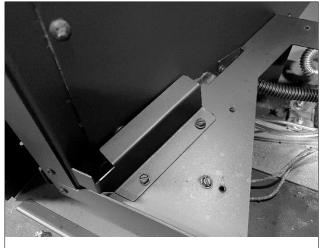
Figure 9.5, Refractory Panel Spacer
