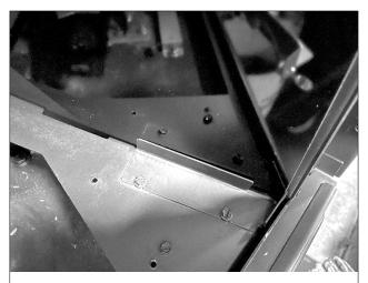
Figure 9.6, Black Glass Bottom Refractory Clip
