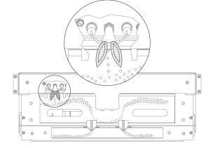
FIGURE 13.2 Correct Burner and Pilot Flame Appearance
