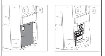
FIGURE 8.12 Control Board Access Cover
