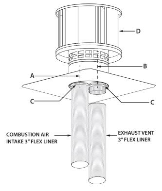
USES #816 36 ft (10.97m) EXPANDABLE 3" FLEXIBLE PIPE
