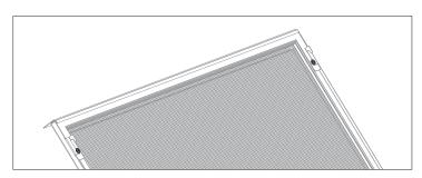
REPLACE (2) SCREWS THROUGH THE HOLES IN THE MOUNTING TAB AND HEAT DEFLECTOR
