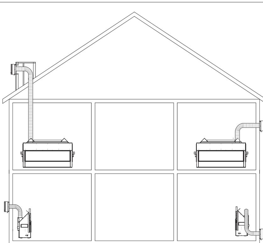
Figure 1.1, Possible Air Duct Locations/Terminations
