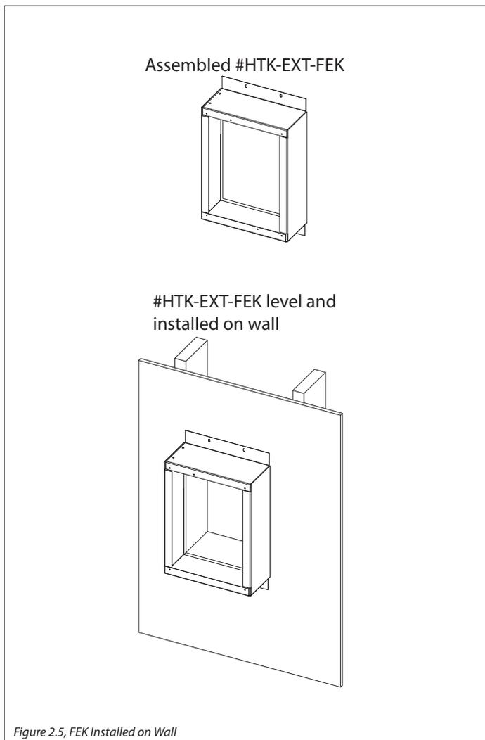
Figure 2.5, FEK Installed on Wall
