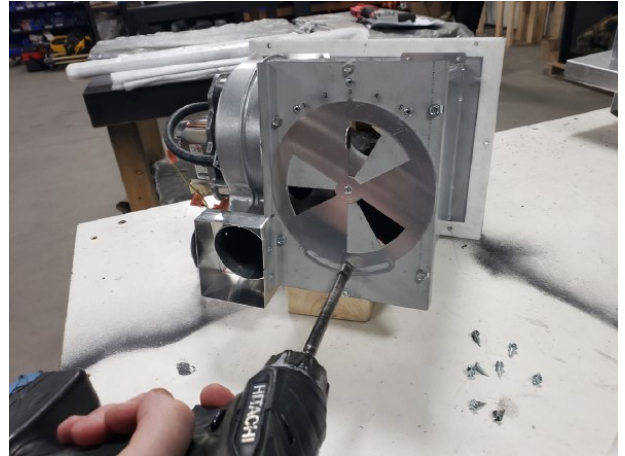
Figure 2.4 - Loosen Locking Screw
