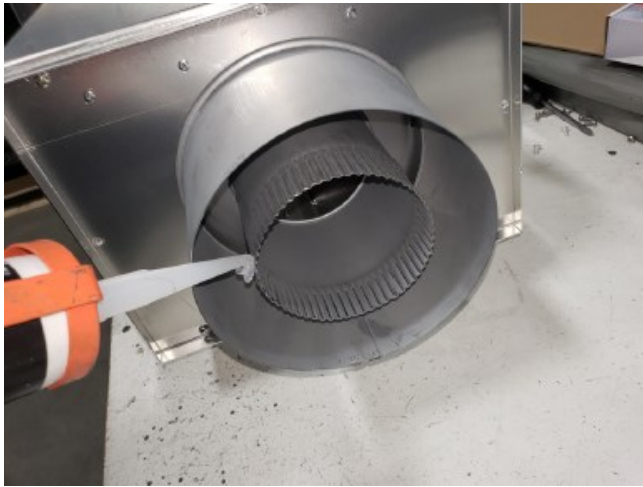
Figure 6.9 - Silicone Inner Exhaust on Power Vent Assembly
