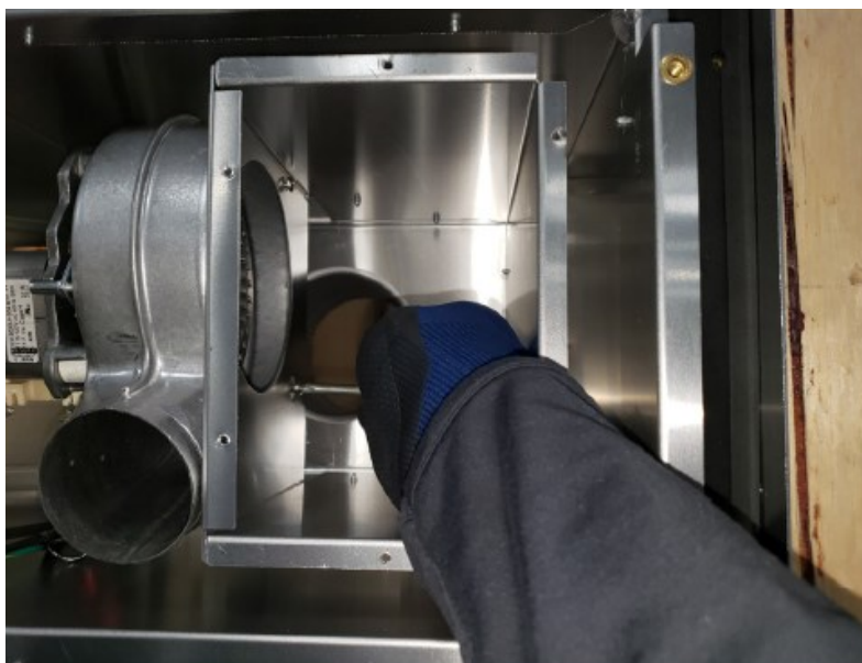
Figure 8.6 - Remove (3) Screws Securing Fan Assembly
