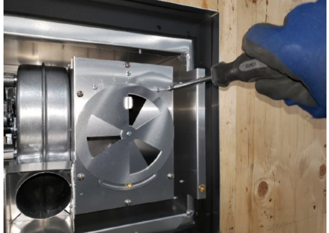
Figure 8.2 - Exhaust Assembly Screws
