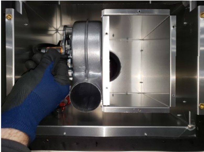
Figure 8.5 - Remove Vacuum Tube
