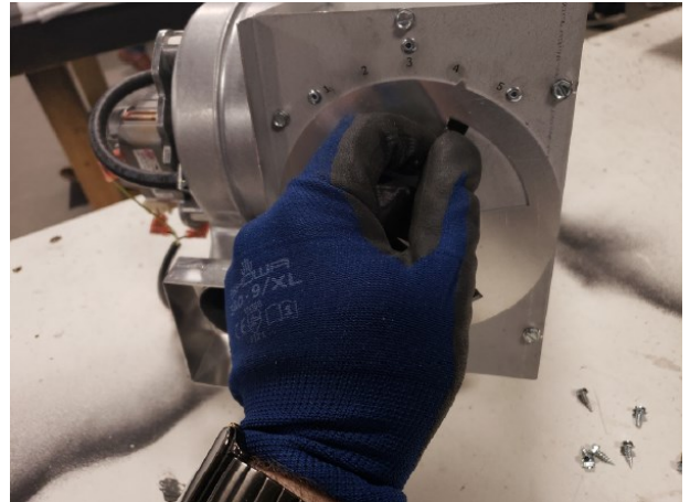
Figure 2.5 - Adjust the Draft Bypass
