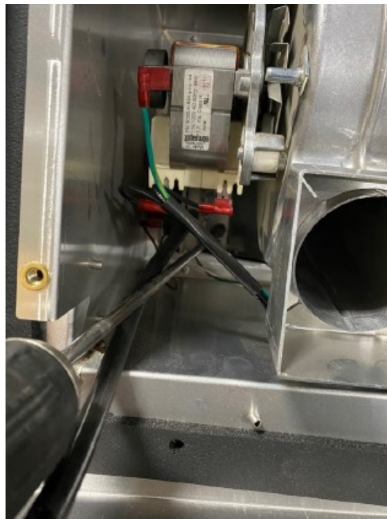
Figure 8.9 - Vacuum Switch Removal
