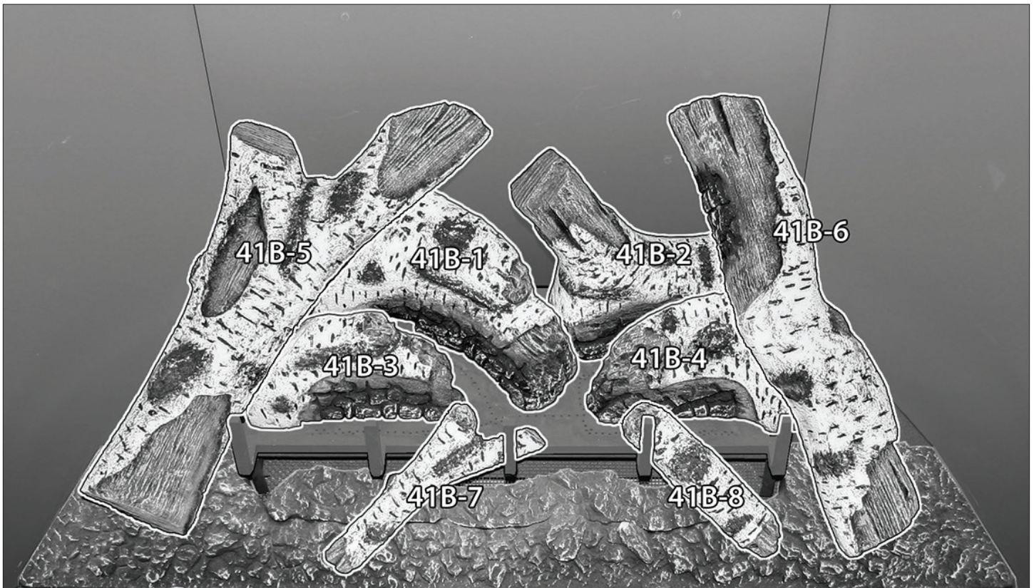
Figure 1, #B41-B501 Log Set Installation
