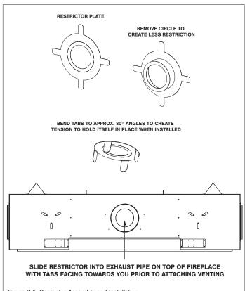
Figure 8.1, Restrictor Assembly and Installation
