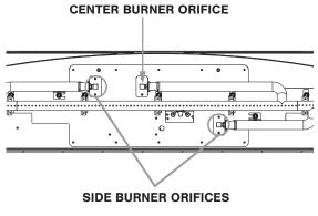
Figure 14.1, Burner and Pilot System
