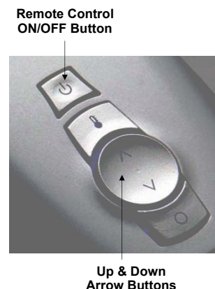
Figure 15.12, Remote Control Functions for System Lockout
