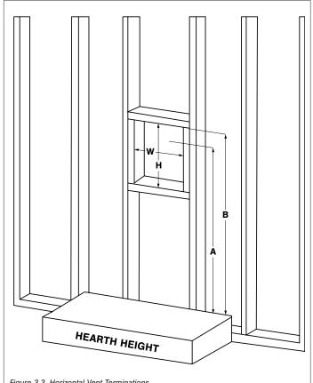
Figure 3.3, Horizontal Vent Terminations
