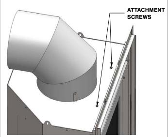
Figure 7.5, Attachment Screw Location
