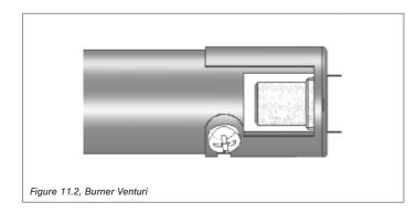
IMPORTANT: Slight adjustments to the venturi opening will create dramatic results. Adjust at slight increments until desired look is achieved. Always burn the fireplace insert for at least 15 minutes, and allow the appliance ample time to cool before making any further adjustments.
