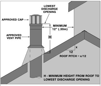
Figure 6.1, Vertical Vent Cap Clearance
