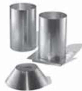
Attic Insulation Shield - Used for installations that pass through an attic. Note: In Canada, Attic insulation shield does not provide sufficient clearance - 3" is required.
